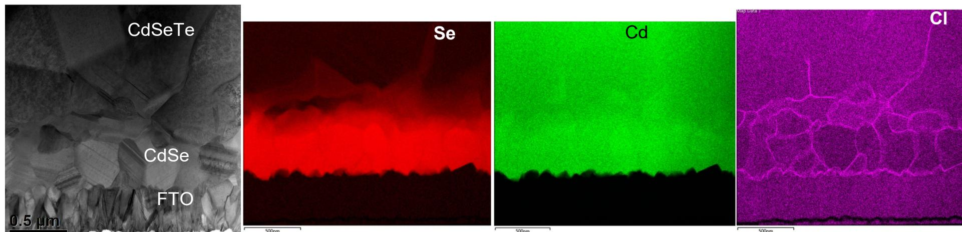
Chlorine present in the CdSe (and CdSeTe) grain boundaries
