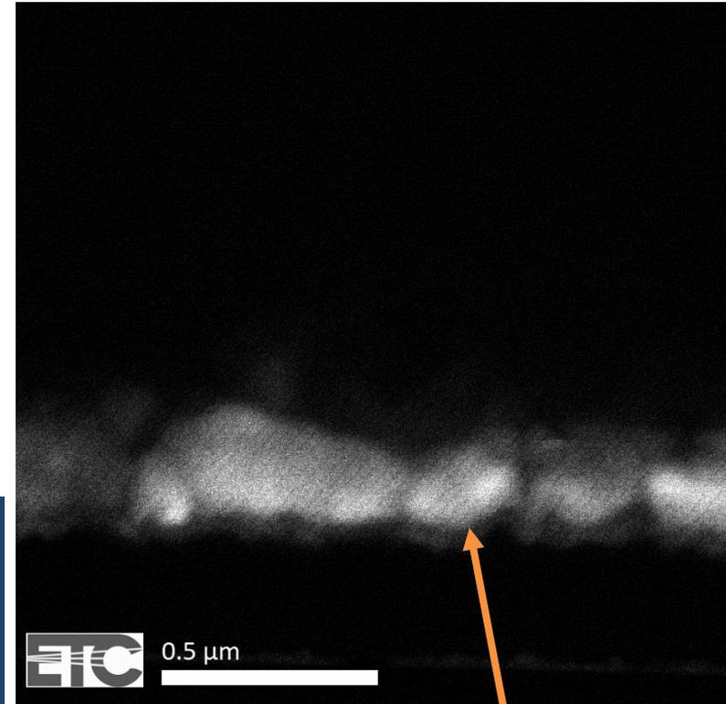
~50 times more intense CL signal in hexagonal CdSe region that has not been fully consumed than CdTe
