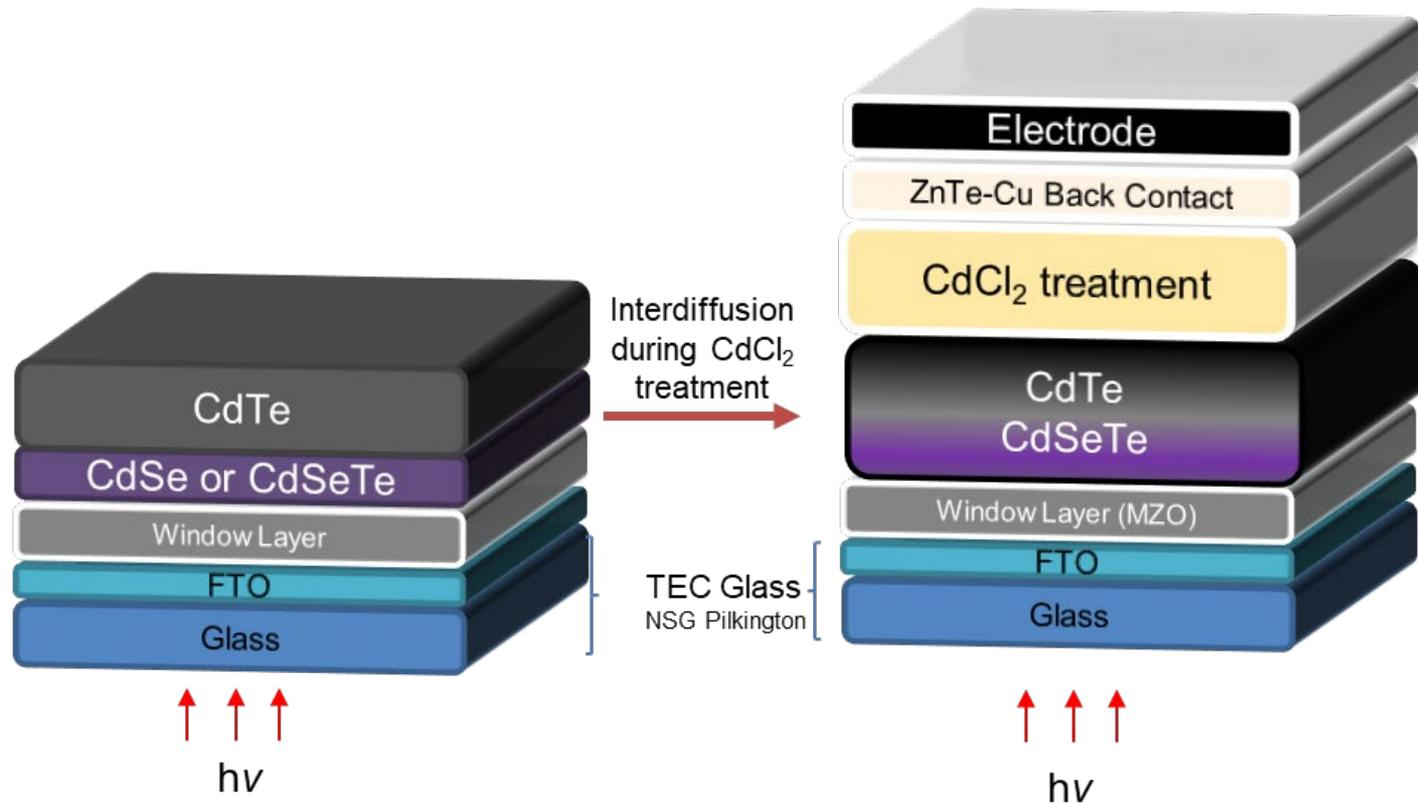
Either CdSe or CdSeTe deposited followed by CdCl<sub>2</sub> used to form absorbers
