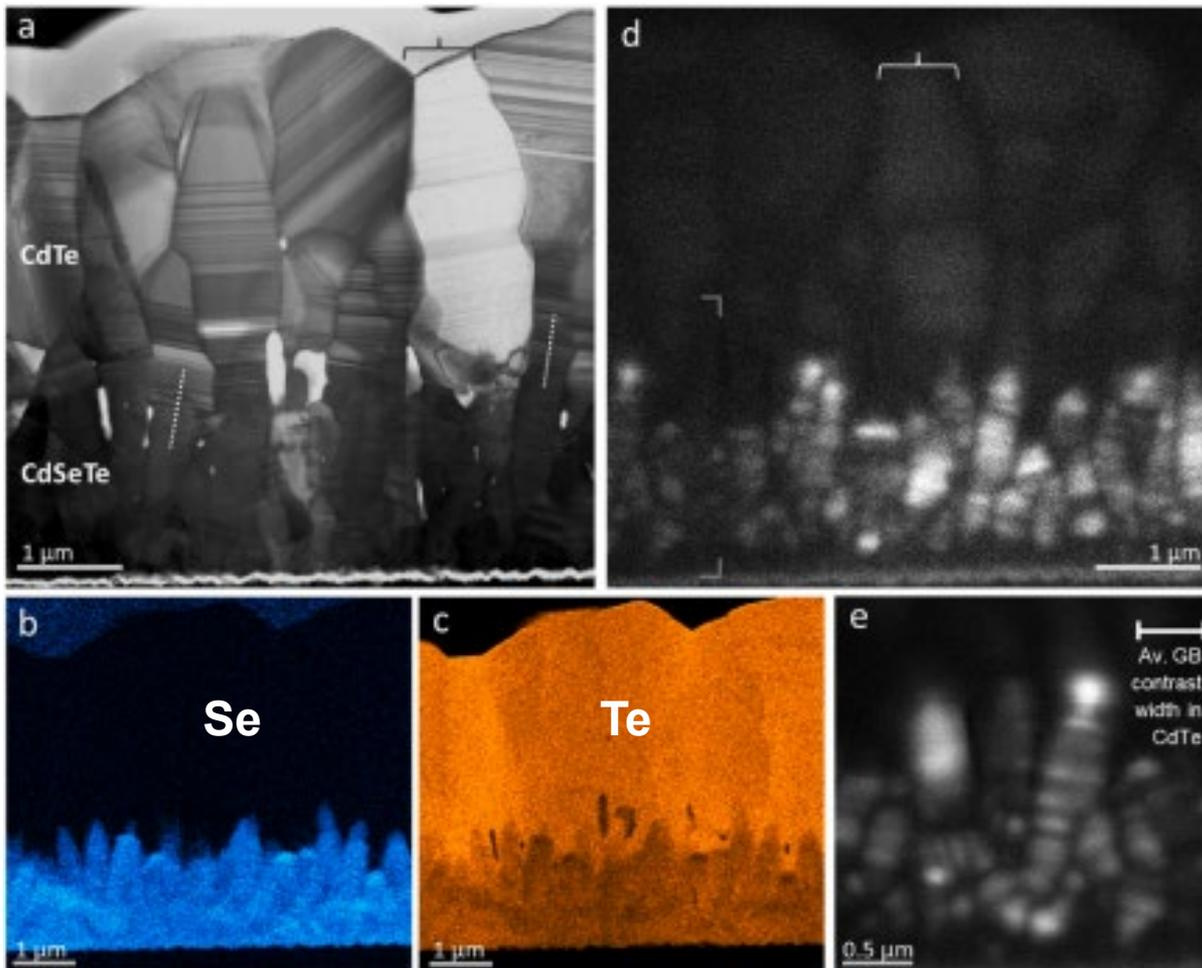
Some CL signal seen from CdSeTe without chloride treatment
