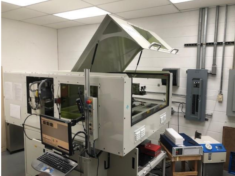
TSI's R&D laser ablation facility accommodates full size 2'x4' PV panels on glass.
