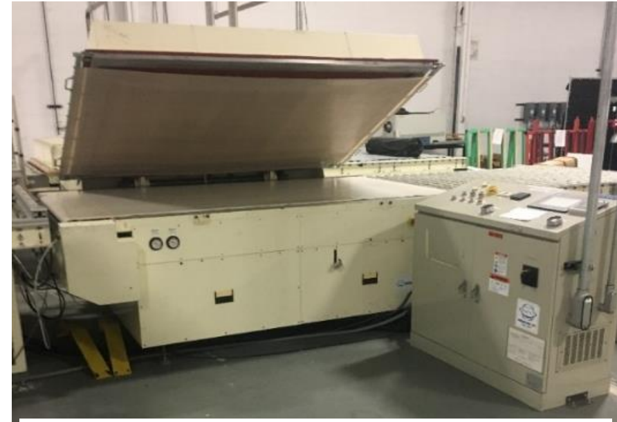
TSI's R&D laminator handles glass up to 4'x6' or three 2'x4' PV modules simultaneously.
