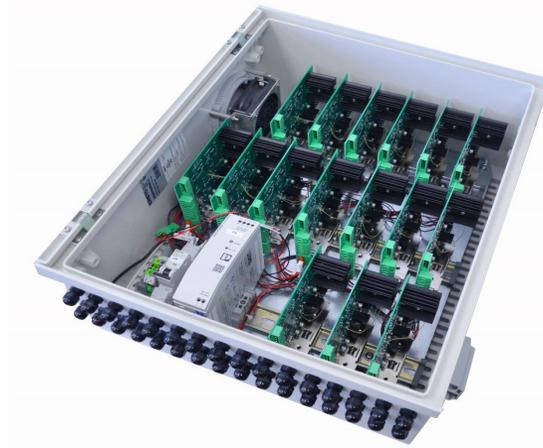
16 measurement/load channels per enclosure, integrated power supply, and computer will provide a complete testing unit.
