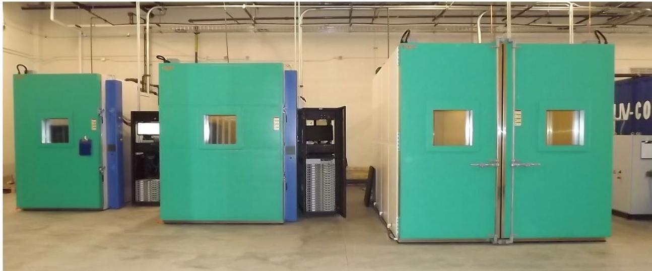
ESPEC Temperature and Humidity Environmental Chambers
