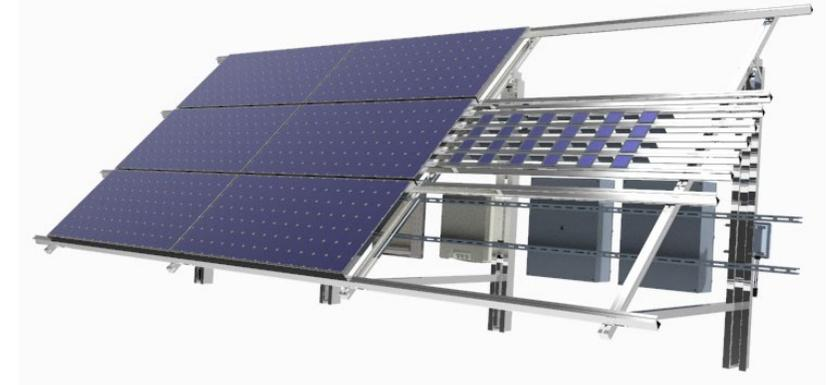
CFV Labs outdoor test rack equipped with irradiance sensors, weather station, and electronic loads specifically designed for mini-modules and cells.
